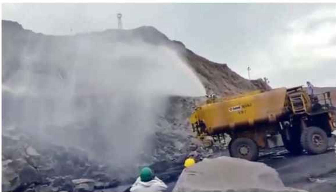
Dust Suppression - Robotics Nozzle at Lakhanpur at MCL
